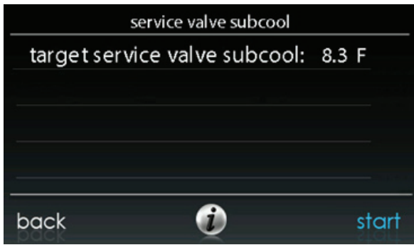
Fig. 11 - Liquid Line Subcooling Target
