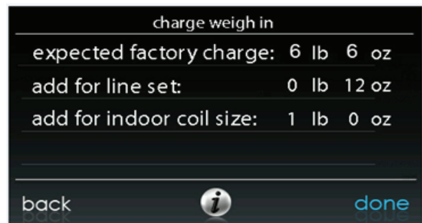
Fig. 10 - Required Charge Adjustment Calculated in UI
